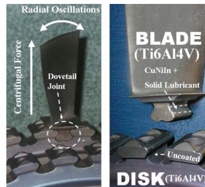
Figure 62: Dovetail joint of blade / disk [231].
