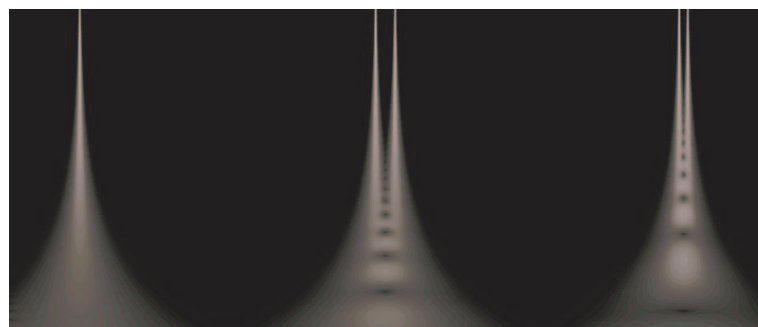
Figure 3.16. Wavelet transform of a signal containing 5 delta-pulses. The distance between two pulses on the right is only 8 ms.
