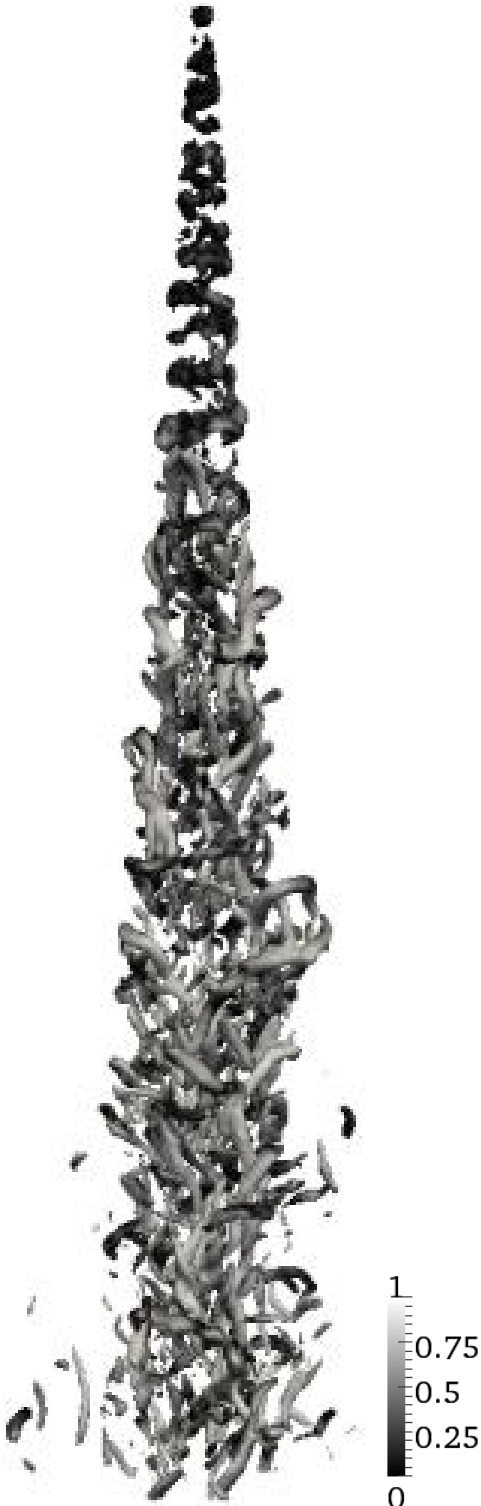
Figure 48: Iso-surfaces of Q_n=0.25 colored by helicity
