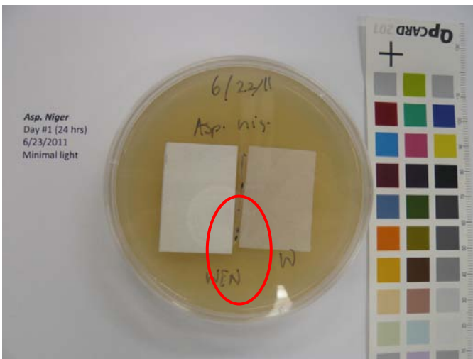
Fig. 8.6 Petri dishes with paper samples were inoculated with Aspergillus niger , along one side, in the center, between the paper samples, marked here with red oval.
