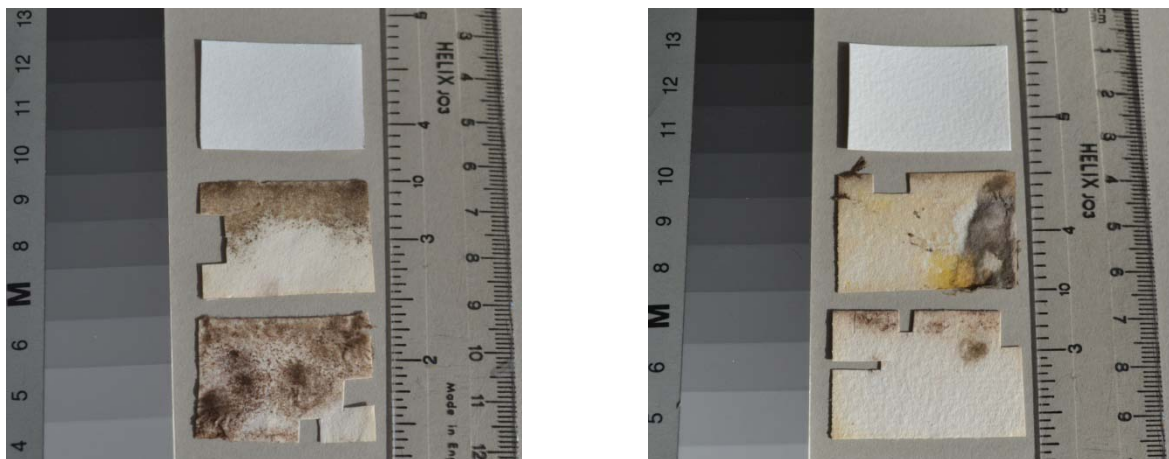
Fig. 2.33 and 2.34 Whatman4 (W4) paper on the left, with fungal pigmentation produced by Aspergillus niger cultured in light and dark conditions.
