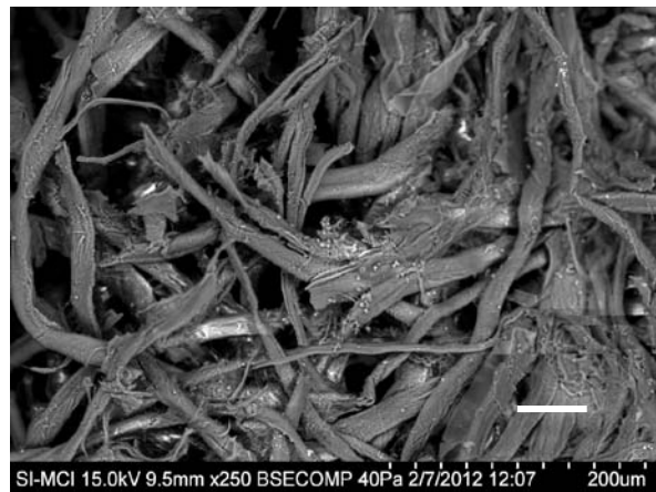
Fig. 2.47 and 2.48. Paper matrix of Whatman4 control (fig.2.47) before inoculation of fungus and after cultivation with A. niger , cultured in daylight. Fig.2.48 shows a physico-chemical deterioration of fibers. SEM-VP micrograph. Scale bar: 50µm
