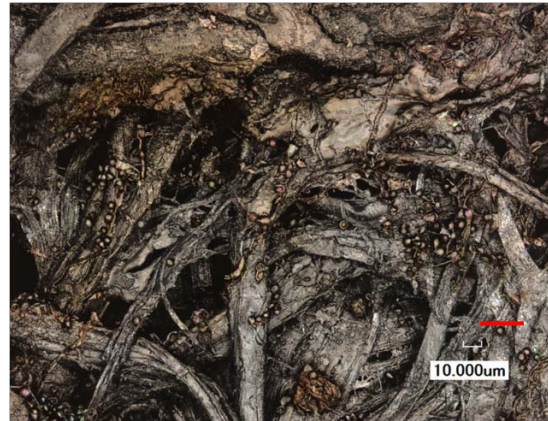
Fig. 9.25 Using short-wave lasers and pinhole optics, a lateral resolution of 0.13 µm 0.01 mm can be obtained. Scale bar: 20 µm
