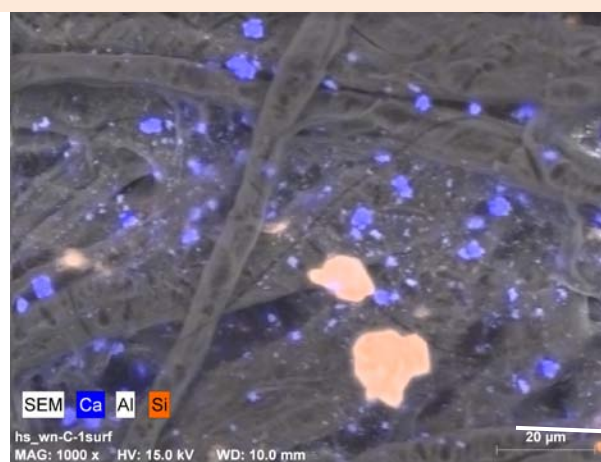
Fig. 8. 42 SEM-XRD elemental analysis confirmed the chemical composition of calcium compound. scale bar: 20 μm
