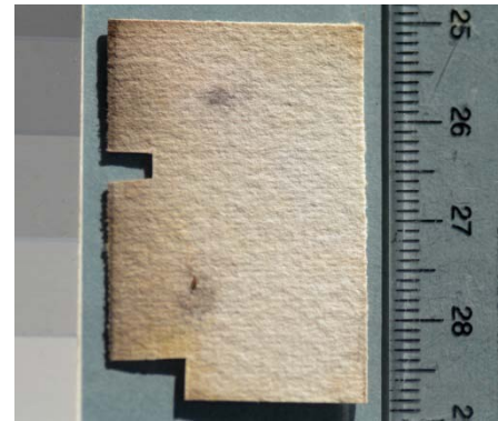
Fig. 8.21 Verso of paper, side facing agar gel. Pigmentation was secreted to paper in areas where colonies grew on recto. Two dark stains corresponded to the growth of colonies on recto.
