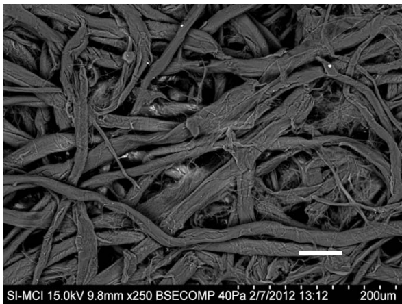
Fig. 2.47 and 2.48. Paper matrix of Whatman4 control (fig.2.47) before inoculation of fungus and after cultivation with A. niger , cultured in daylight. Fig.2.48 shows a physico-chemical deterioration of fibers. SEM-VP micrograph. Scale bar: 50µm
