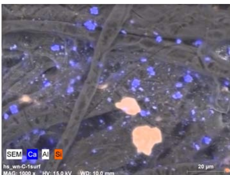
Fig. 2.49-51. Calcium carbonate filler in Winsor&Newton paper was modified by biogenic activity of Aspergillus niger to calcium oxalate. SEM-VP with EDS analysis confirmed the same chemical base composition with main component calcium, however of different crystalline configuration.
